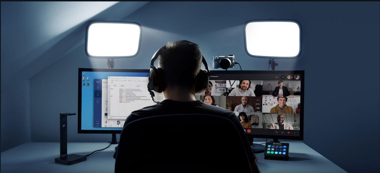
When using more than one Key Light, position them on either side of your desk, aimed at your face at a 45-degree angle. This is the best way to properly illuminate a green screen or wall that is behind you, and eliminate shadows that would be created by a single light source. Key Light features adjustable brightness and color temperature, so you can set ideal lighting conditions for your workspace.
